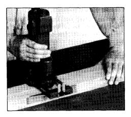
Install the straight guide on the guide holder with the wing bolt. Then use the hex wrench to loosen the bolts on the tool base and insert the guide holder into the grooves in the tool base. Adjust the distance between the bit and the straight guide and tighten the bolts securely. When adjusting the straight guide up or down, loosen the wing bolt. After adjusting it, tighten the wing bolt securely.
